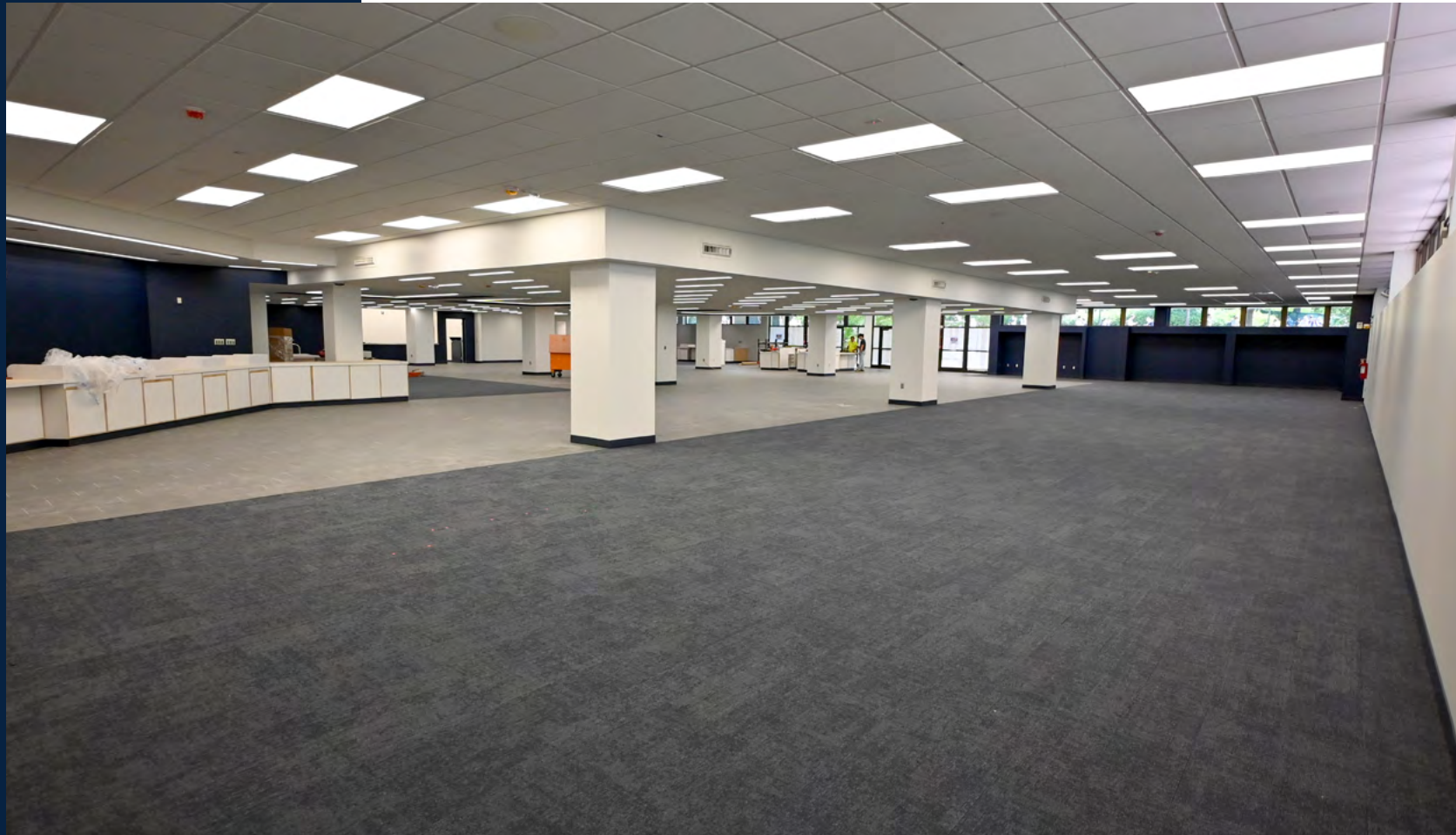
The main retail sales floor includes new recessed LED lighting to replace the previous fluorescent lighting.
