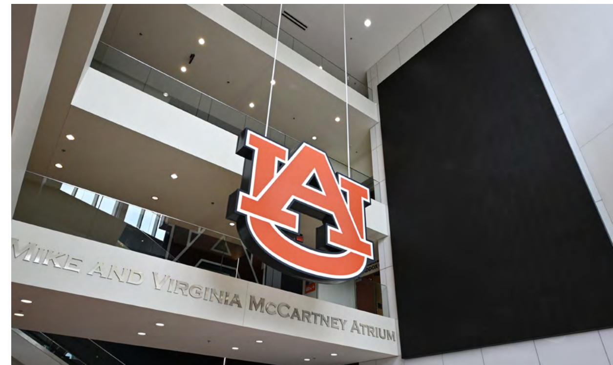
The new Daktronics LED atrium display is 34x18 feet and weighs about two tons. It is made from five different LED video displays.
