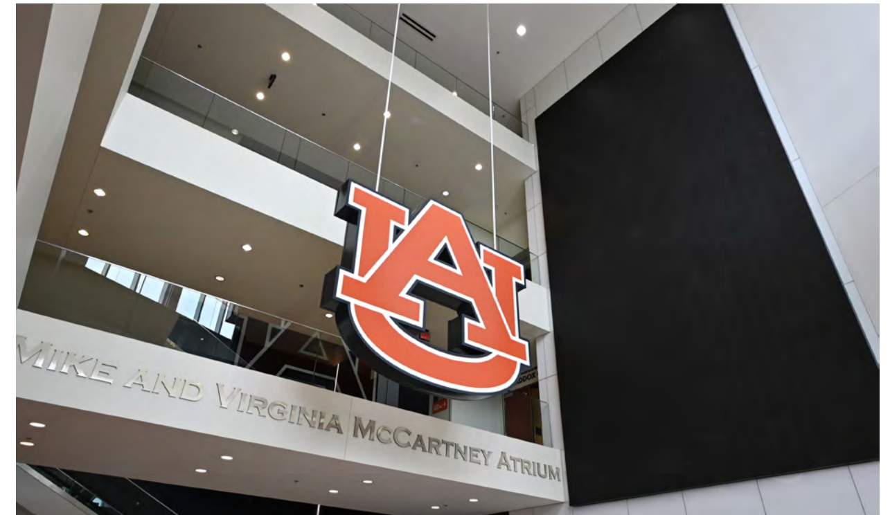
The new Daktronics LED atrium display is 34x18 feet and weighs about two tons. It is made from five different LED video displays.
