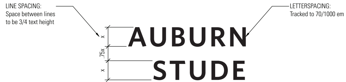
5 Detail: Spacing Scale: 1 1/2" = 1'-0"
